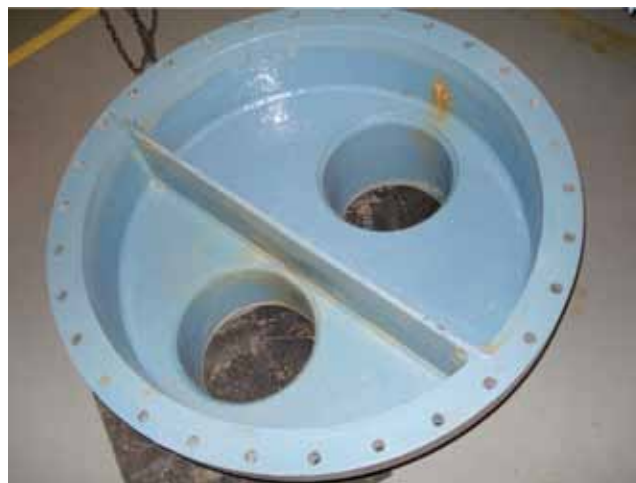
▲ Figure 7. An epoxy coating on mild-steel tubesheets (top) and water boxes (bottom) prevents the buildup of iron rust deposits that could break off and plug tubes, and eliminates galvanic corrosion.
